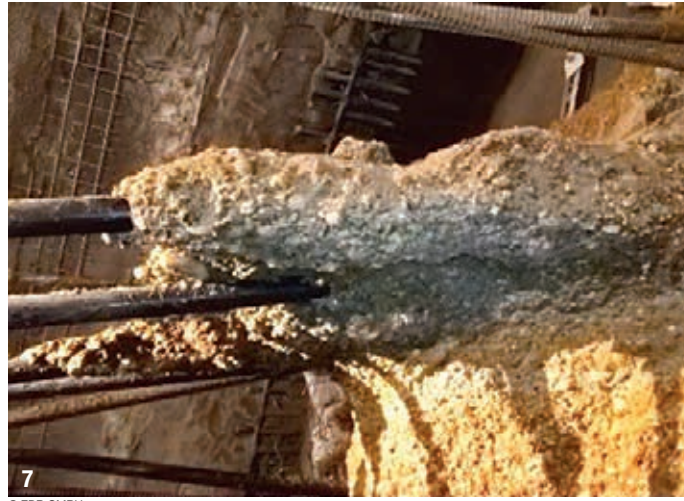
7- Test section for acrylic injected soil. 8- Aerial view of main shaft.
