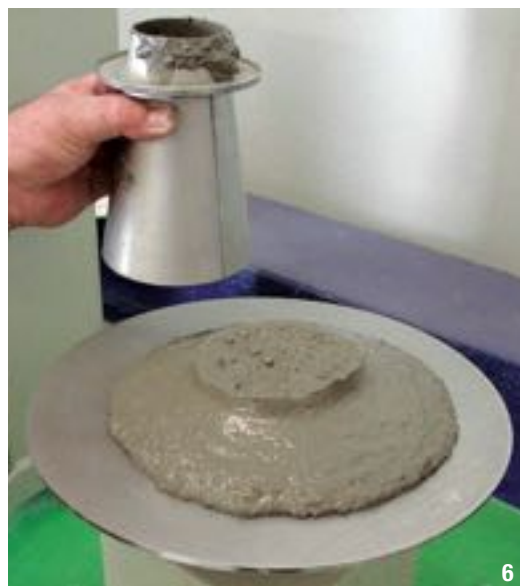
7- Illustration of the fresh mortar's cohesion just after consolidation tests (water extraction) at 1 bar for half an hour.
