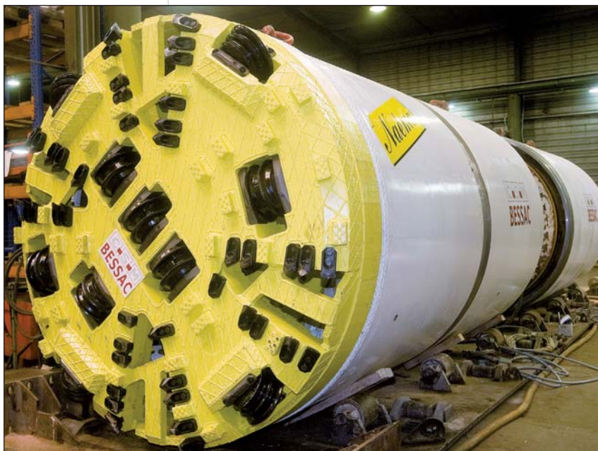
Photo 3 Microtunnelier en usine Microtunnel boring machine in factory
