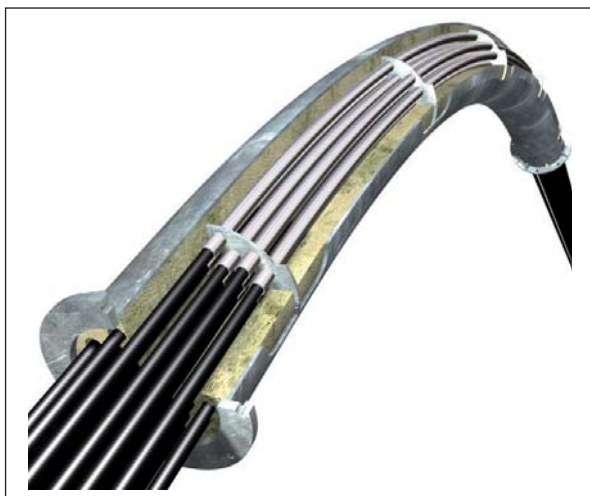
Figure 1 Écorché de la selle multitube Phantom view of the multitube saddle
