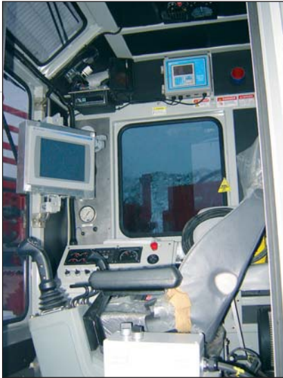
Figure 11 Foreuse Cubex QXW 810 : vue de la cabine Cubex QXW 810 Drill – View of Operator Cabin
