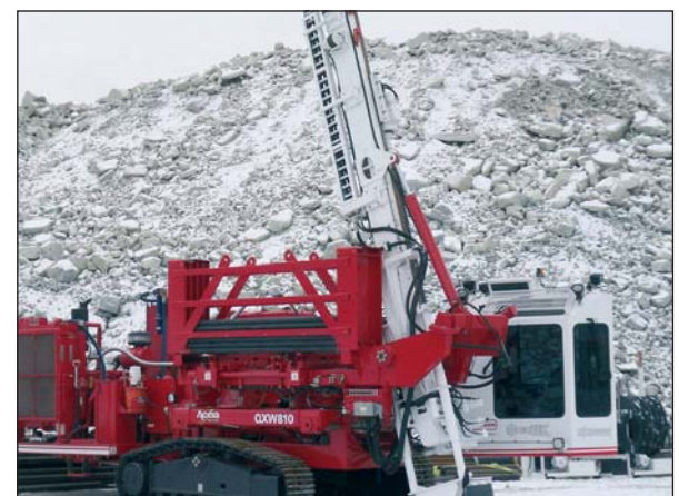
Figure 10 Foreuse Cubex QXW 810 Cubex QXW 810 Drill
