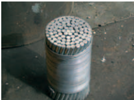
Photo 10 Fabrication des haubans TMC Manufacture of TMC stay cables
