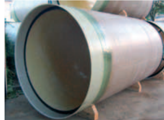
Photo 7 Le tuyau de fonçage en PRV 1600 mm The driving pipe in 1600 mm GRP
