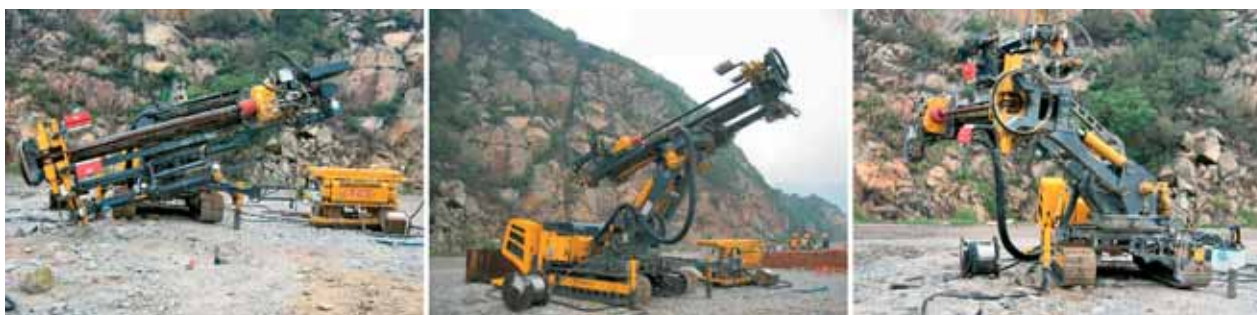
Photo 2 Quelques positions possibles de la MEDIAN Some possible positions of the MEDIAN
