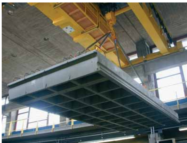
Cellular slab in ultra-high- performance fibrous concrete for composite bridge. National project MIKTI – LCPC – Paris
