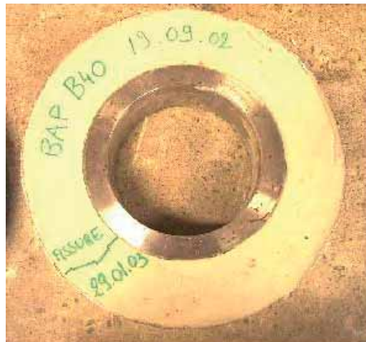
Photo 8 Anneau de fissuration Cracking ring
