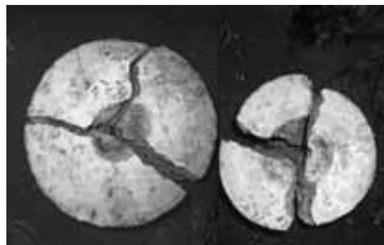
Figure 9 Failure of split test specimens
