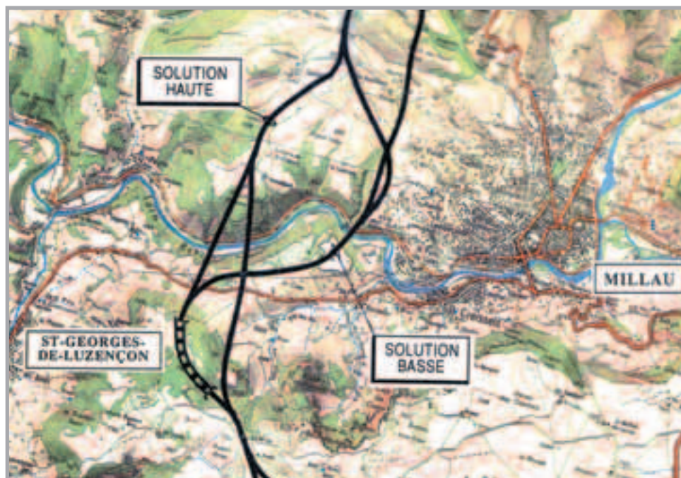
Figure 10 Tracé des solutions haute et basse Layout of the high and low solutions
