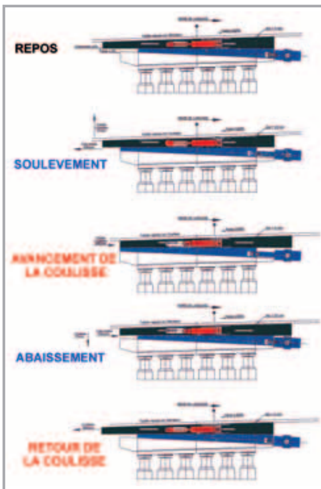
Figure 12 Principe de translation du tablier Schematic of deck translational movements
