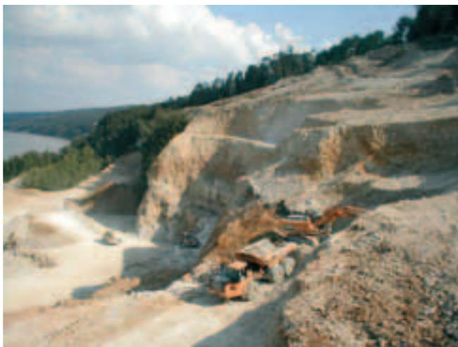
**The start of operations. Creation of stepping. In the background along the Seine, one can see very clearly the sensitive botanical area (presence of a rare fern) which forced 25 % of the pit bank area to be frozen (machinery manoeuvring zone)**
