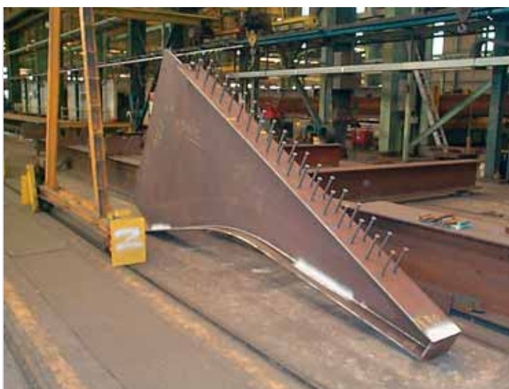
Photo 7 Console en cours de fabrication Cantilevered beam during manufacture
