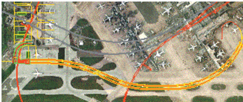
Photo 4 Tracé en plan de l'ART (Airside Road Tunnel) Horizontal alignment of the ART (Airside Road Tunnel)
