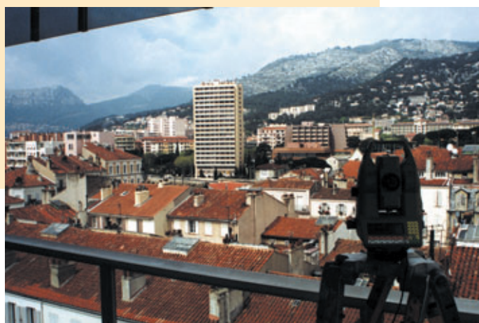
Toulon Tunnel : real-time view of the subsidence basin
