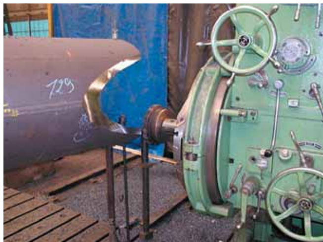
Figure 7 Préparation des chanfreins Preparation of bevels
