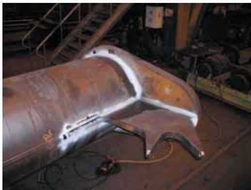
Figure 14 Assemblage platine P3 sur membrure inférieure Assembly of plate P3 on lower member
