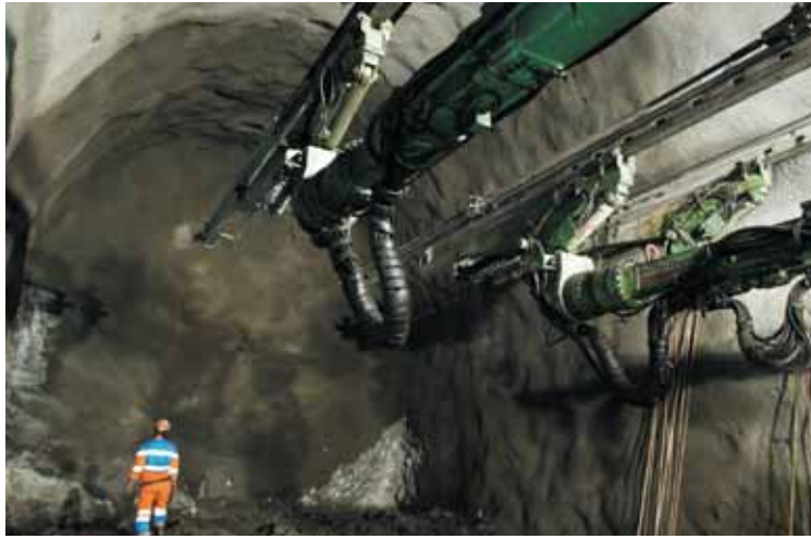
Photo 2 Jumbo de foration trois bras Three-arm jumbo drill
