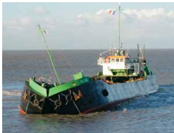
Photo 6 Chaland automoteur lors d'un clapage Self-propelled barge during sediment dumping at sea
