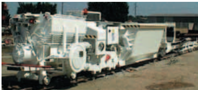
Photo 3 Le train de marinage The mucking train
