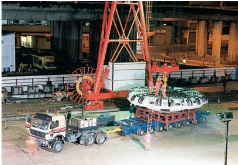
Photo 10 Tunnelier - Assemblage de la jupe TBM - Assembly of skirt
