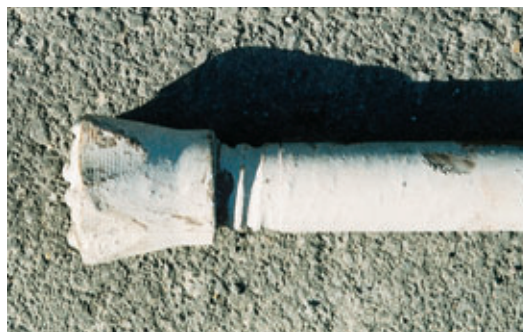
Photo 1 Armature du clou auto-foré munie du taillant perdu Self-boring nail assembly with disposable cutting edge
