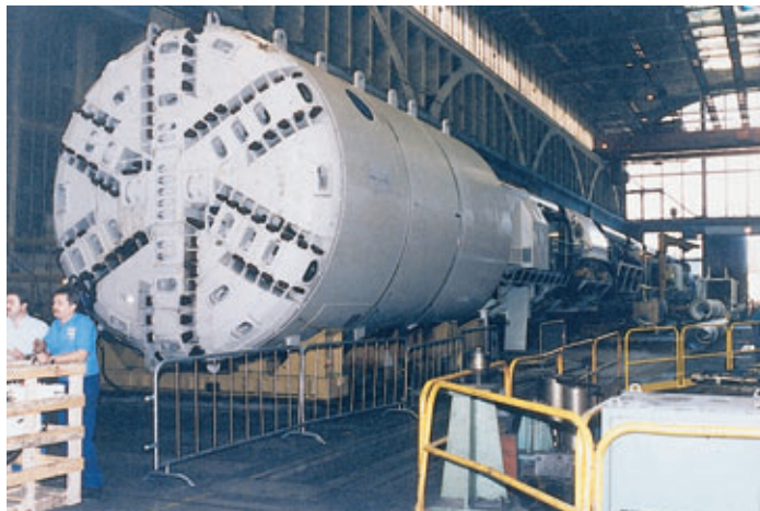
Photo 4 Tunnelier en cours de construction TBM during construction
